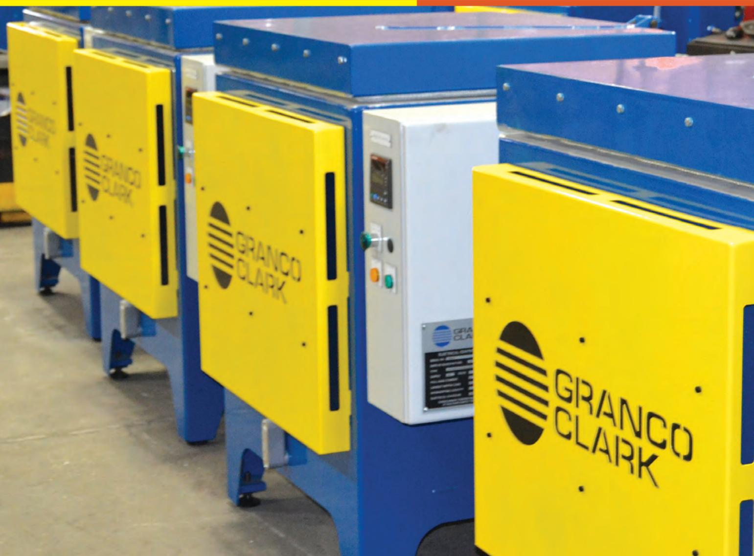
The **GRANCO CLARK** Infrared Die Oven provides the fastest die heating times available. It heats dies uniformly in less than 25 percent of the time required by traditional die ovens. While a typical die for a mid-size press takes approximately four hours in a convection oven, the **GRANCO CLARK** Infrared Die Oven brings the same die to temp in less than 60 minutes.
