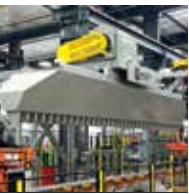
Air Quenching Highest cooling rates available
