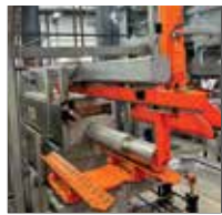
Billet Taper Quench 10% - 40% ram speed increase
