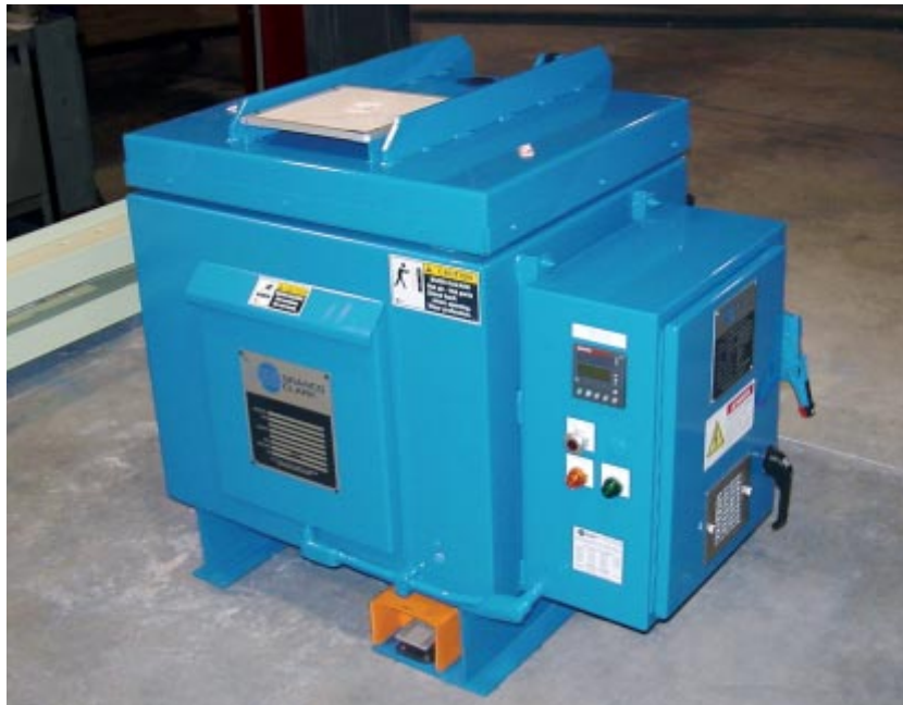
The Granco Clark infrared oven measures the temperature of the die as it is heated, allowing it to be used as a top-off oven for warm dies.
