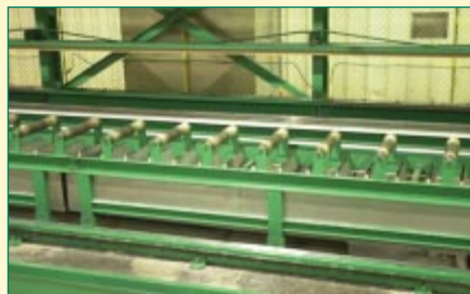
Granco Clark Integral Cooling Duct System
