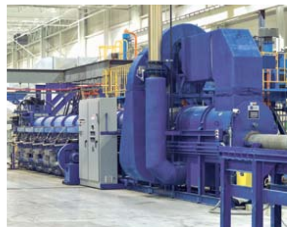
Granco Clark Hot Jet Furnace
