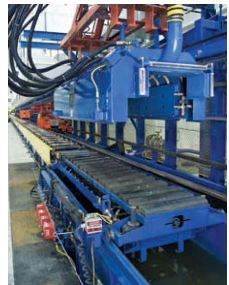
High-pressure spray offers faster quenching...as long as the profiles can tolerate it.
