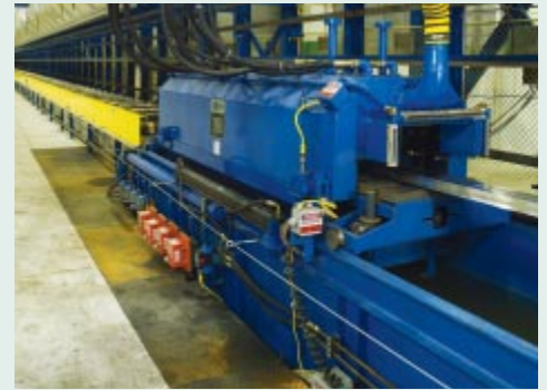
The Granco Clark High-Pressure Spray Quench provides the maximum heat transfer available in a profile quench, so it's capable of cooling even large shapes quickly.
