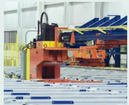
Granco Clark's Controlled Vertical Crush Stretcher delivers maximum gripping control with minimum distortion. The design uses a pivoting upper jaw that can be set to any closing dimension.
